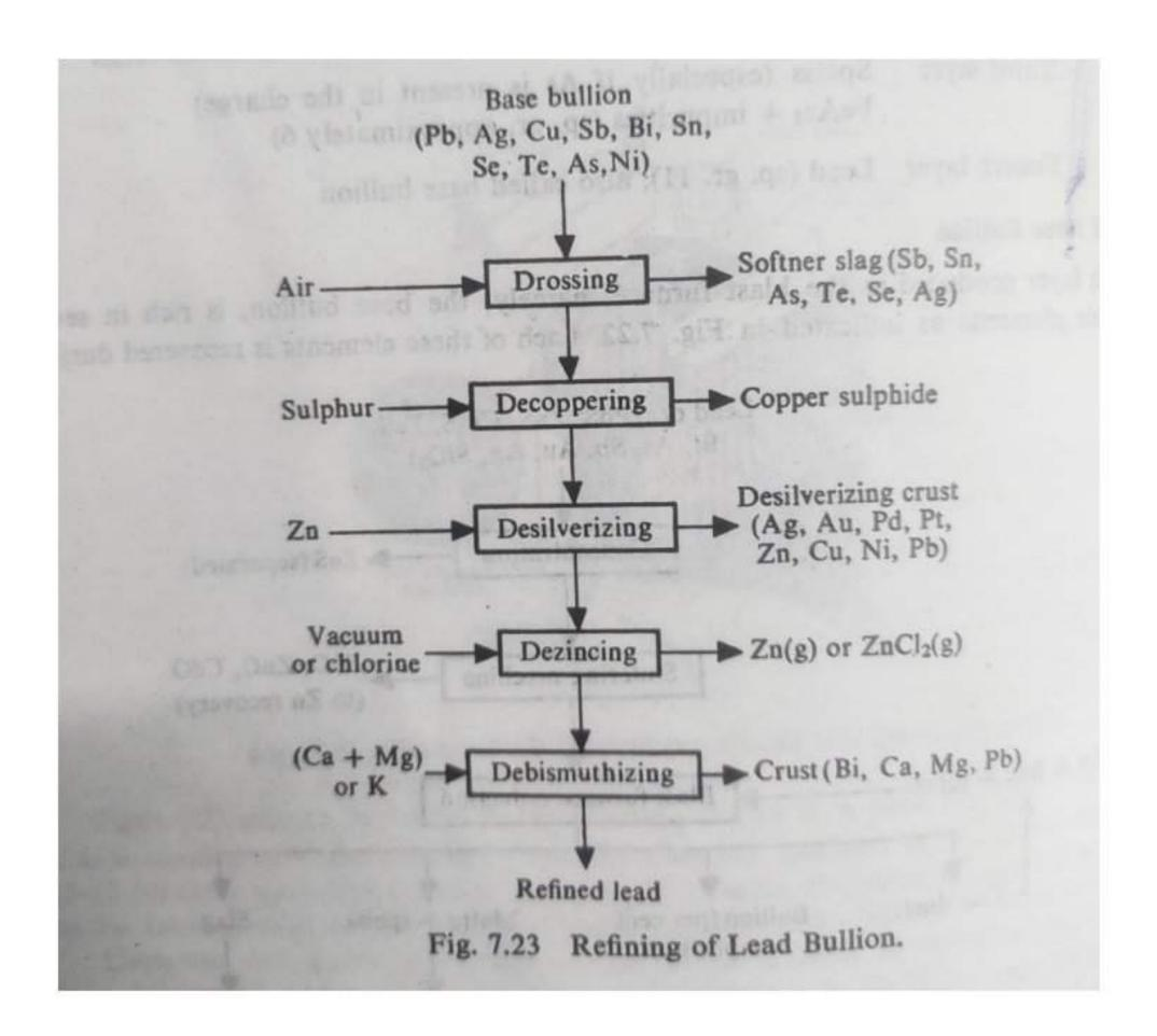
**DROSSING-** Drossing is a combination of liquation & oxidation usually carried out in a reverberatory furnace. Base bullion is first subjected to drossing at around 350°C. At 350°C metals like Sb, Sn, As,Te, etc get oxidised and are skimmed off.
