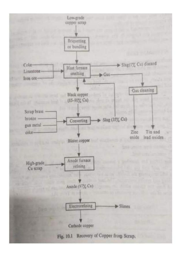
The copper scrap originates from foundaries fabrication and user industries. The breakdown is as follows: dross, spillages and skimmigs from foundaries; punching, tunnlings and brings from fabrications; scrap, cable, wires radiators from cars, buses, bronze, brass from user industries. The scrap dealers sort out the scrap accordingly to the grade & composition.
