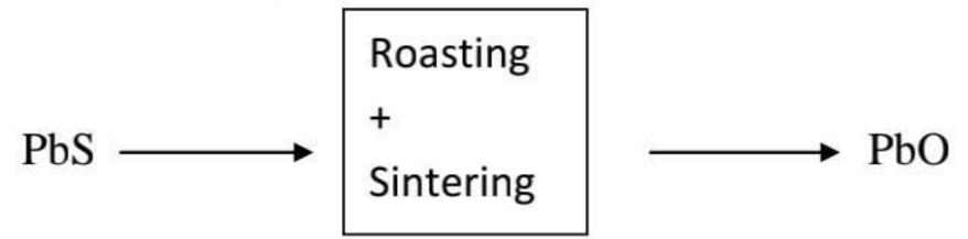
During roasting, the concentrated ore roasted to oxides which is subsequently reduced by carbon & temperature must be control because above 800°C PbS tends to fuse.
