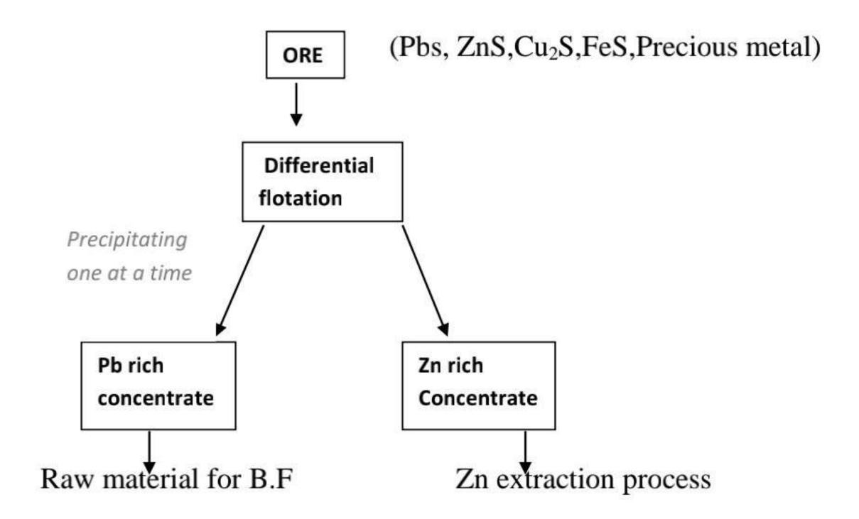
The ore Galena (PbS) is grind into fine powdered so as to increase surface area for extraction of lead. The main aim of concentration is to remove impurities. The lead ore contains lead sulphide with other sulphide & precious metal. The lead sulphide along with precious metal is fast separated from other sulphide and is concentrated by differential flotation process. The concentrate may contain 60-80% Pb.
