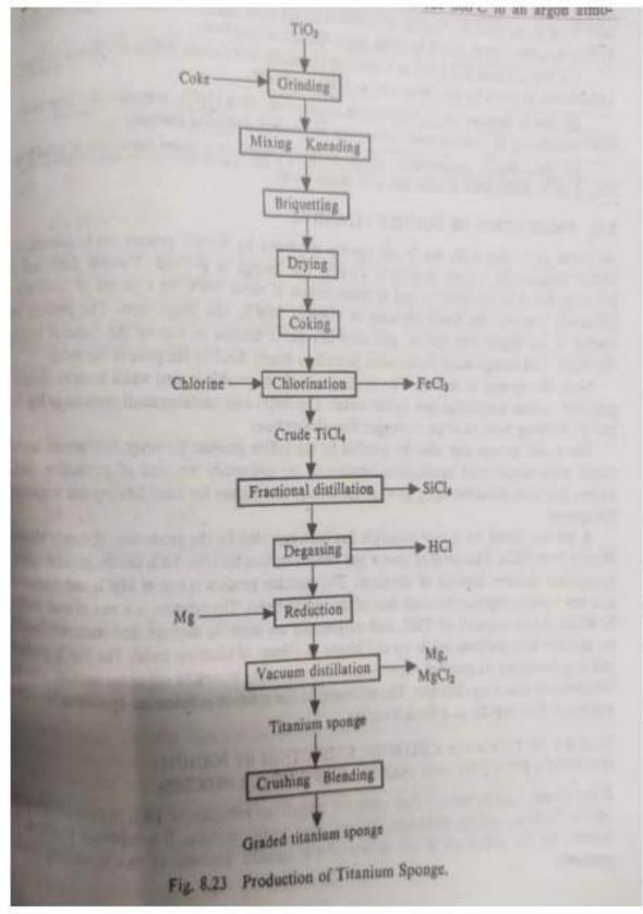
The residue is a pure titanium sponge. Several precaution have to be taken during reduction. The reduction chamber has to be first heated to a high temperature of about 900°C and flushed with hydrogen to eliminated all oxygen in order to avoid the oxidation of magnesium. All possible MgO coating is thus removed and temperature is lowered to 800-850°C.
