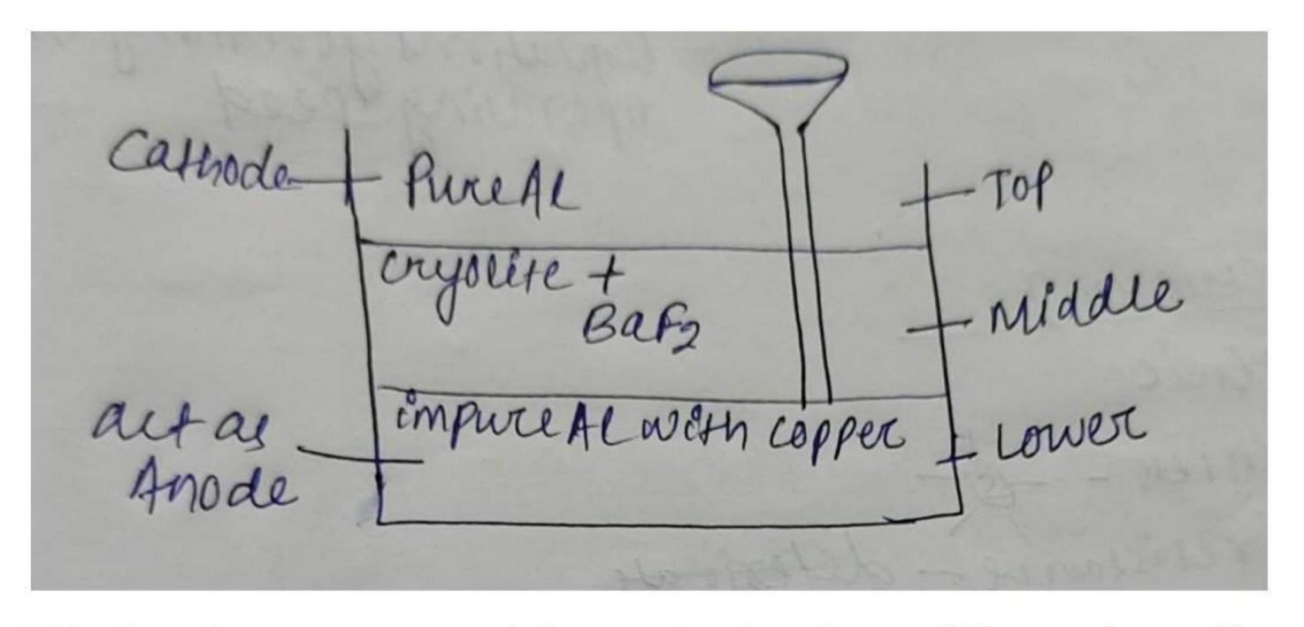
This three layers are separated form each other due to difference in specific gravity.
