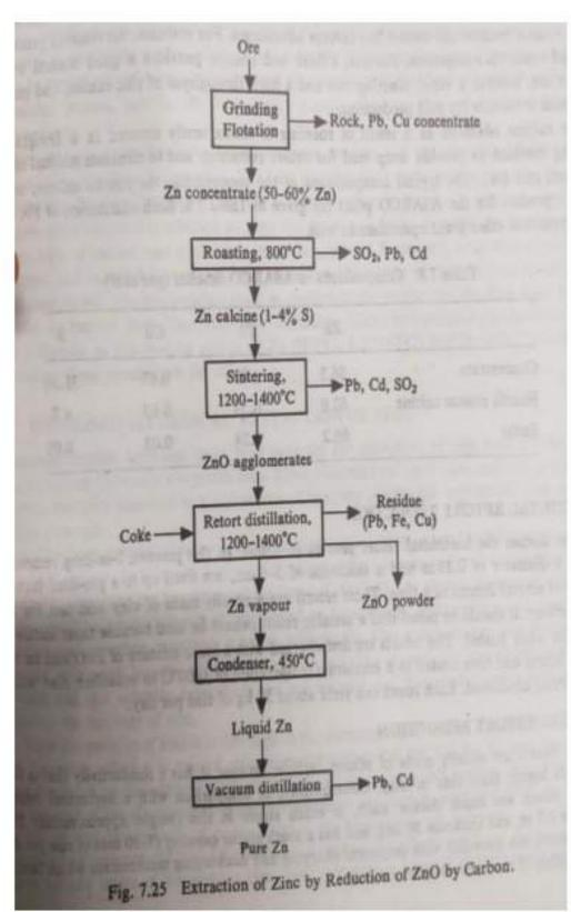
The resultant roasted oxide is first ground and agglomerated and then sintered at 1200°C so as to provide a feed in the form of lump for retort reduction.
