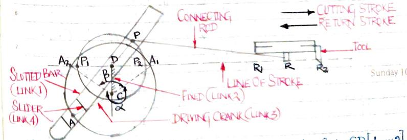
In this type of shaper machine mechanism, the link CD [LINK 2] forming the turning pair is fixed as shown in the above figure. The link 2 matches to a crank in a reciprocating steam engine. The driving crank
