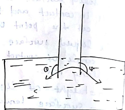
(Q) calculate the capillary rise in a glass tube of 2.5 mm diameter when immersed vertically in (a) water and (b) mercury. Take surface tension  $\sigma = 0.0725 \text{ N/m}$  for water and  $\sigma = 0.52 \text{ N/m}$  for mercury in contact with air. The specific gravity for mercury is given 13.6 and the angle of contact =  $130^\circ$ .
