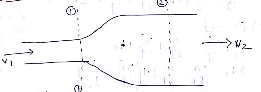
Consider a liquid flowing through a pipe which has sudden enlargement as shown in above figure. consider two sections ①-① and ②-② before and after enlargement.
