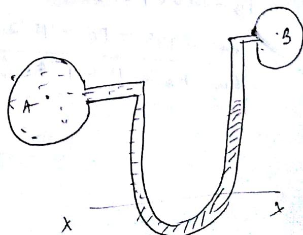
Q) A differential manometer is connected at the two points A and B as shown in figure. At B air pressure is  $9.81 \text{ N/cm}^2$ . Find the absolute pressure at 'A'.
