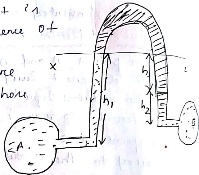
Q) A differential manometer connected at the two points A and B of two pipes containing air. The pipe A contains a liquid of specific gravity = 1.5 while pipe B contains a liquid of sp. gravity = 0.9. The pressures at A and B are 1 kgf/cm<sup>2</sup> and 1.80 kgf/cm<sup>2</sup> respectively. find the difference in mercury level in differential manometer.
