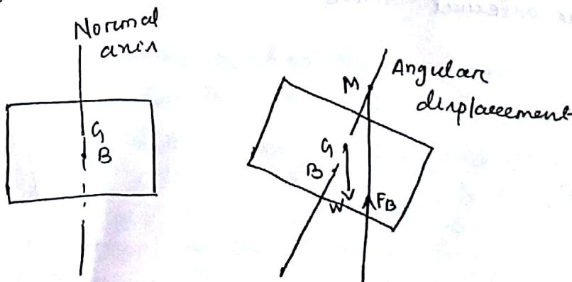
→ It is defined as the point about which a body starts oscillating when the body is tilted by a small angle.
