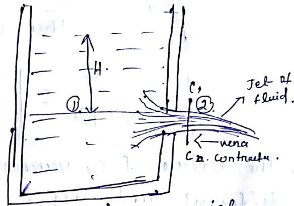
① coefficient of velocity ( $C_v$ ) :- It is defined as the ratio between the actual velocity of jet of liquid at vena contracta and the theoretical velocity of jet.
