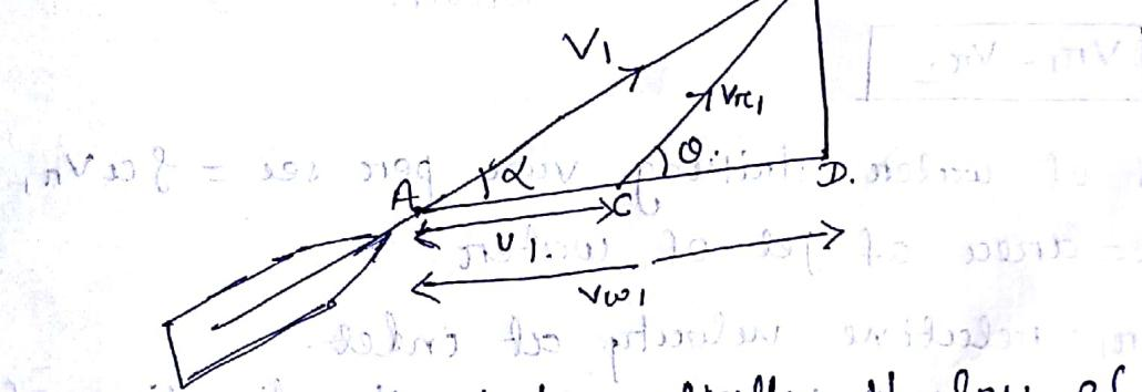
→ As the ~~jet~~ jet strikes tangentially, the loss of energy due to impact of the jet will be zero. as the plate is moving, the velocity with which jet of water strikes is equal to the relative velocity of the jet with respect to the plate.
