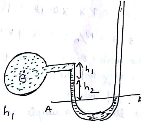
(Q) (1) Simple U-tube manometer containing mercury is connected to a pipe in which fluid of sp. gravity 0.8 and having vacuum pressure is flowing. The other end of the manometer is open to atmosphere. Find the vacuum pressure in the pipe if the difference of mercury level in the two limbs is 40cm and the height of fluid is 15cm. left from the centre of pipe is 15cm. below.
