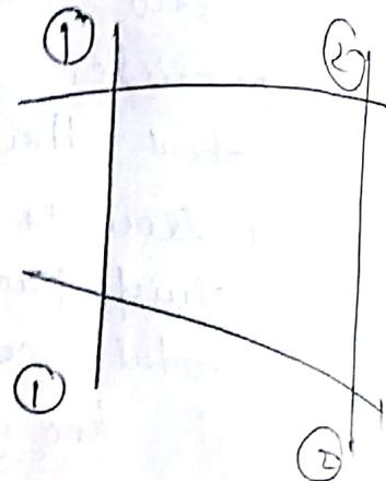
Q) A 30cm pipe containing water, branches into two pipes of diameters 20cm and 15cm respectively. If the avg. velocity in the 30cm pipe is 2.5m/s find the discharge in the pipe. Also determine the velocity in 15cm pipe if the avg. velocity in 20cm pipe is 2m/s.
