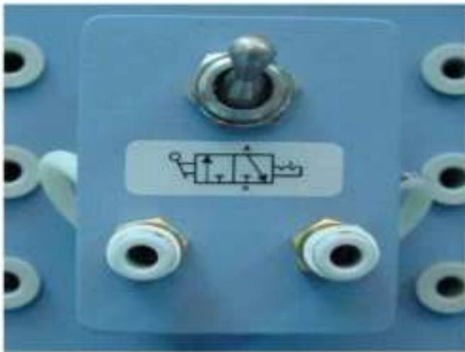
Fig. 10 (a) 3/2 directional control valve (b) Cross section
