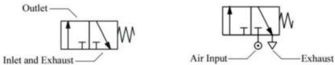
Fig 17 3/2 directional control valve (normally closed type)
