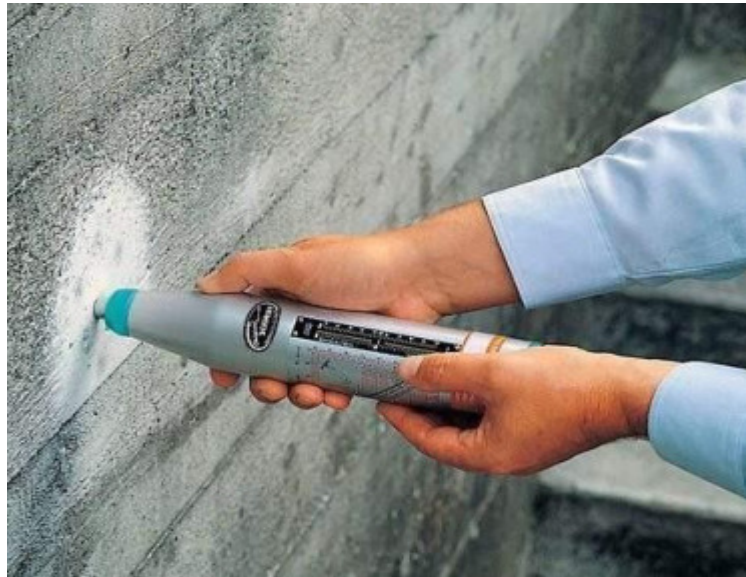
NDT test on concrete
