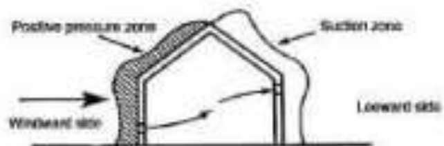
Wind pressure diagram for roofs with pitches above 30°
