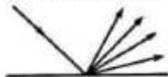
Light scattered and reflected from a semi-matt surface
