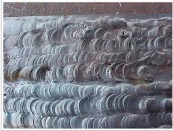
Figure 7.23 unacceptable weld profiles
